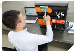
快速瞬变脉冲群抗干扰实验 Anti-interference test of fast transient pulse group
