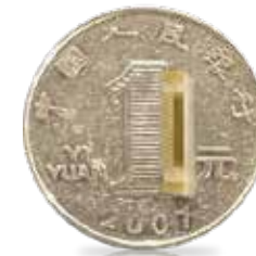
一元硬币及32线集成光学发射芯片 One yuan coin and 32-line integrated optical emitting chip
